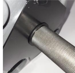
If dial lock is hard to move, unscrew bolt slightly. Dial lock should move but not be loose.
